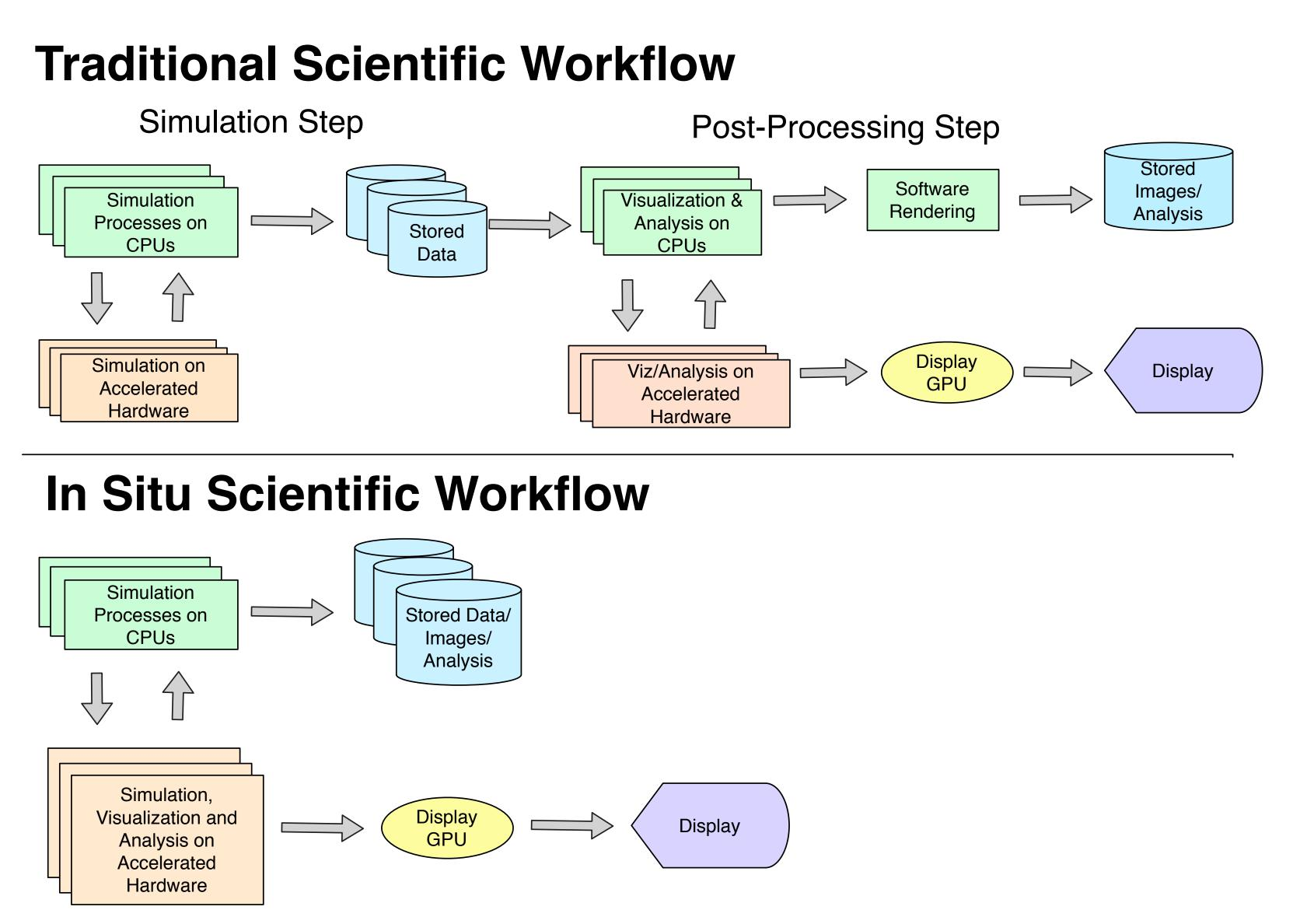
Figure 1. Post-processing model vs. In Situ via Scout
